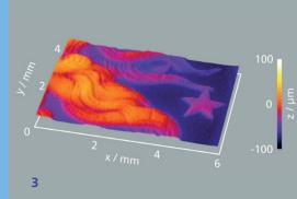
HoloTop detects the topography of surfaces quickly and reliably enough for inline inspections.
