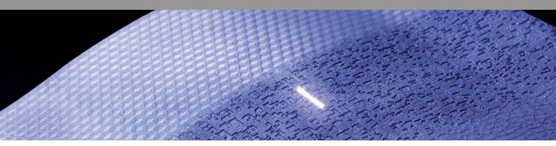
Adaptive laser based micro structuing of complex surfaces
