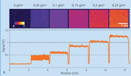
a high area throughput with simultaneous high sensitivity. The signals detected are combined to form a spatially resolved overall image. Thanks to its collimated laser beam, the system features a considerable depth of field. Beside its application for monitoring rollstock, the system also allows reliable detection of critical points on complex components.
