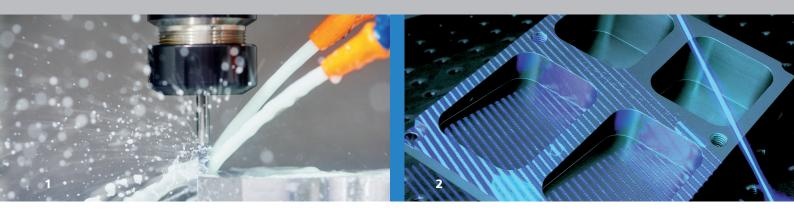
1+2 A fluorescence imaging measurement system by Fraunhofer IPM detects contamination or defects on surfaces directly in the production line.
