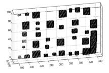
GFRP A-sandwich specimen with a foam structure\* with various internal defects. Sample size (mm): 340 x 200; defect size (mm): 6 x 6 to 25 x 25. Right: result of automatic defect detection.
