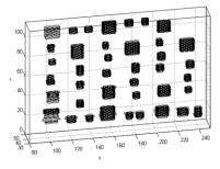
GFRP C C-sandwich specimen with a honeycomb structure\* with various internal defects. Sample size (mm): 340 x 200; defect size (mm): 6 x 6 to 25 x 25. Right: result of automatic defect detection.
