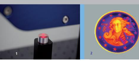
HoloTop detects the topography of surfaces quickly and reliably enough for inline inspections.
