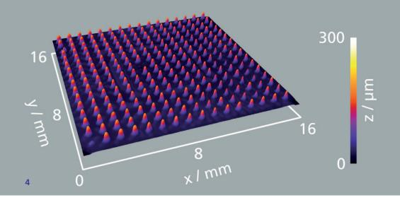
limeter range, depending on roughness. The measurement resolution and reproducibility depend on the distances between the individual wavelengths used and the surface properties of the object and can be adapted to the specific application.
