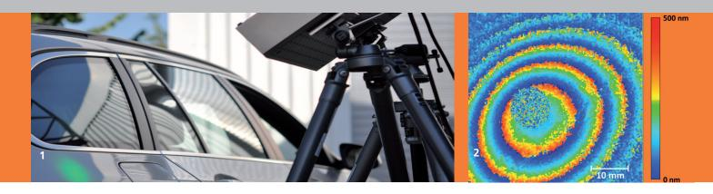
The ESPI system from Fraunhofer IPM is robust and portable. Here, thermal deformation of a car body is measured.
