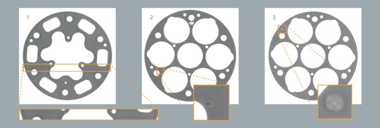
**1-3** Scratch, blister, and dent as defect examples; the gaskets are represented at a scale of approximately 1:2.
