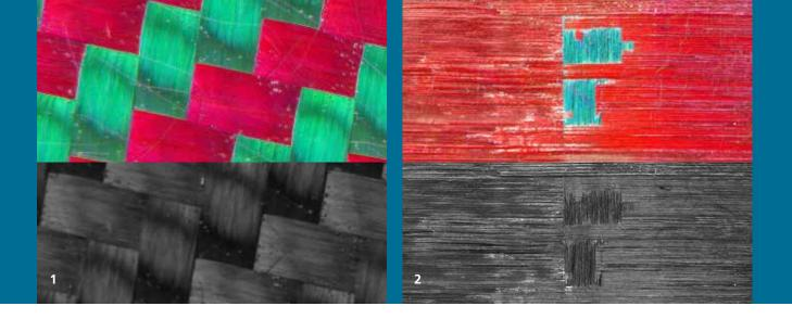
light parallel to the direction of the fiber. Our camera exploits this effect to determine which way the fiber runs.
