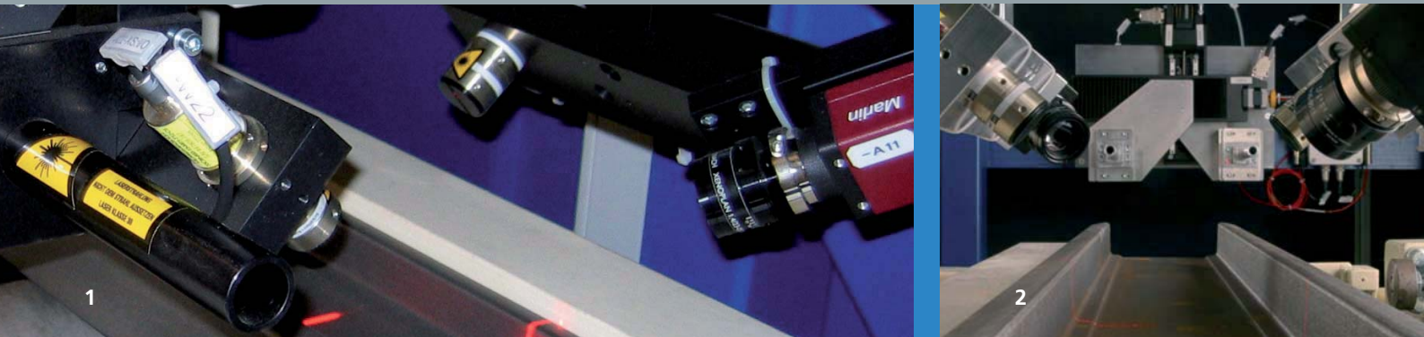
1, 2 Sensor unit for straightness inspection. Photos: Fraunhofer IFF
