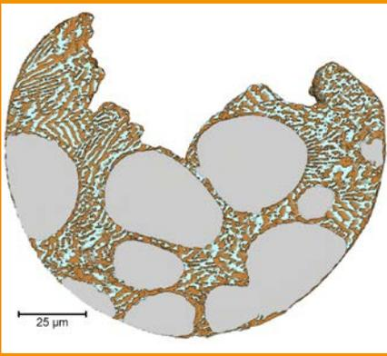
**2** Section parallel to the YZ plane of the segmented data (Avizo Fire); the  $\alpha$ -aluminum phase is shown in gray, the aluminum in the eutectic is light blue, and the  $Al_2Cu$  intermetallic phase is shown in dark orange.
